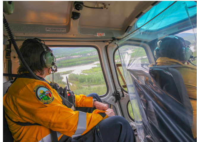
Plexiglass dividers were installed in helicopters to reduce contamination during flights.
