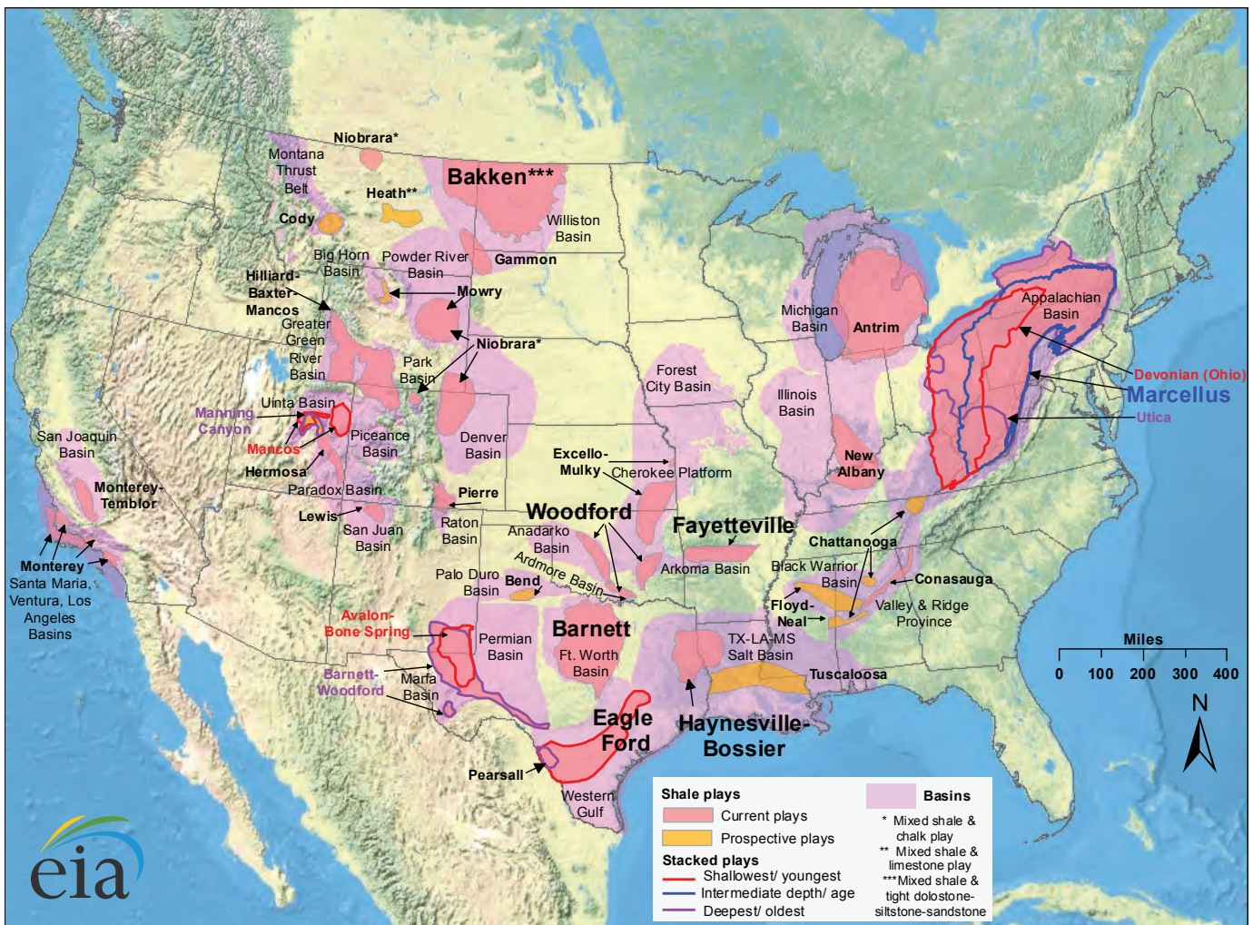
Figure 10. Shale gas basins and play trends, continental United States (from U.S. Energy Information Administration, 2011b).
