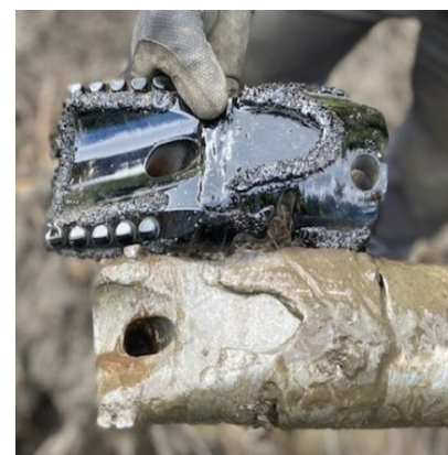
Photo of a new and used drill bit after encountering hard rock
